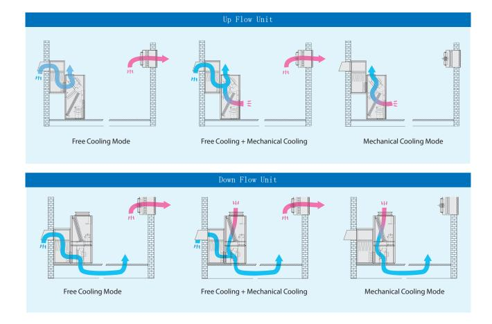
OPTIMA-INV-DFC systems include mechanical (DX) cooling and free cooling modes, together with the intelligence to switch between the modes to ensure the most efficient operation. When utilizing direct free cooling, the DX system compressor stops, which has a significant impact on the energy consumption.
