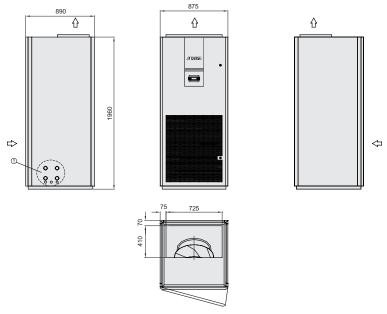
① Pipe connect area: Specific position and kinds differ slightly in different unit series. Refer to the onsite unit.
