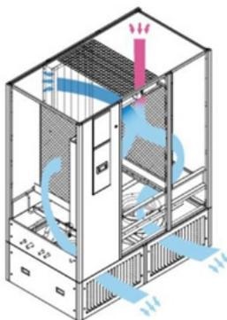
During periods of extreme low outdoor temperatures, the return air damper will modulate to temper the outside air with warmer inside air. This is to maintain design supply air temp in low ambient conditions.
