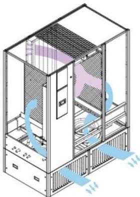
When the outside ambient temperature is above 20°C the adiabatic function is activated. The units' own internal intelligent control then monitors the room humidity, and when this pre-set value falls outside of acceptable limits, the adiabatic function is stopped and the room air is extracted until the humidity values fall back inside the programmable limit. The EC fans continue to run to ensure make-up air is still introduced to the room.
