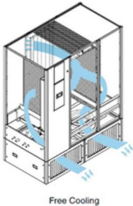
This is the standard optimum cooling mode as the unit utilizes the outside air to cool the room via variable speed EC supply fans. The fan speed modulates with the room cooling demand to provide the most energy efficient method of cooling. When the ambient temperature is 5°C or more below the indoor temperature, fresh air free cooling will supply 100% of the cooling capacity.
